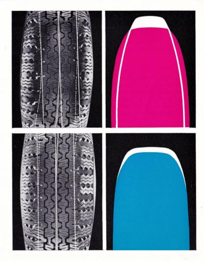
The displacement of contact area in a conventional tyre (top) caused by a sideways force either when cornering or by wind is shown by the white lines. In addition the tread channels close up in the contact area. Pressure: 21 lb Tyre Load: 772 lb, Sideways force: 309 lb.
