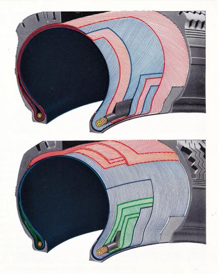
A conventional tyre is composed of several carcass plies of textile, set at opposing angles of approximately 100 degrees to each other and 40 degrees to the tyre centre line. (blue and red)
